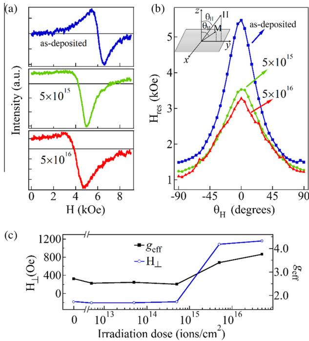
**Fig. 5.** (a) FMR spectra of the as-deposited and irradiated sample with a series of different proton dose when an applied field is normal to thin film. (b)  $H_{res}$  as a function of  $\theta_H$  for the as-deposited and irradiated sample with a series of different proton dose. (c)  $H_{\perp}$  and the  $g_{eff}$  of  $H_{res}$  as a function of proton irradiation dose for NiZn ferrite thin films.
