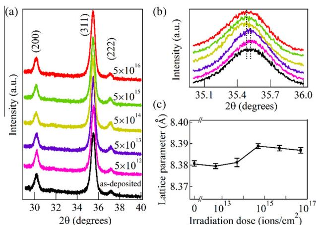
**Fig. 1.** (a) GIXRD patterns of NiZn ferrite thin films for the as-deposited sample and a series of different proton irradiation dose. (b) The (311) peak in detail. (c) The curves of the lattice parameter as a function of proton dose.
