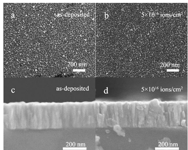
**Fig. 2.** (a) and (b) SEM images of the surface images of the as-deposited and irradiated samples with a dose of  $5 \times 10^{16}$  ions/cm<sup>2</sup> respectively. (c) and (d) The cross-sectional SEM images of the as-deposited and irradiated samples with a dose of  $5 \times 10^{16}$  ions/cm<sup>2</sup> respectively.
