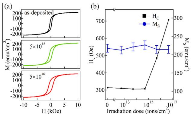
**Fig. 4.** (a) The in-plane magnetic hysteresis loops of the as-deposited and irradiated samples with a series of different proton dose. (b)  $M_s$  and  $H_c$  as a function of proton dose. The circle and square dots represent  $M_s$  and  $H_c$ , respectively.
