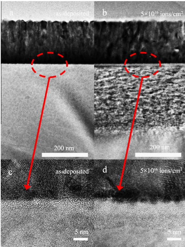
**Fig. 3.** (a) and (b) the cross-sectional TEM image of the as-deposited and irradiated samples with a dose of  $5 \times 10^{16}$  ions/cm<sup>2</sup> respectively. (c) and (d) High-resolution cross-sectional TEM image of the as-deposited and irradiated samples with a dose of  $5 \times 10^{16}$  ions/cm<sup>2</sup> respectively.
